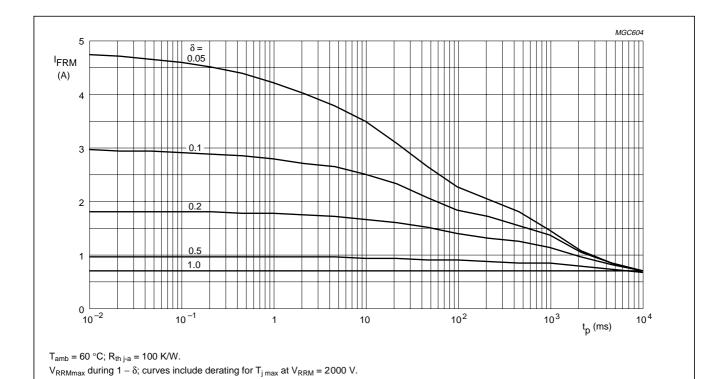
Fig.5 Maximum repetitive peak forward current as a function of pulse time (square pulse) and duty factor.
